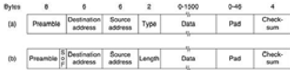
Figure 10-5. Frame formats. (a) DIX Ethernet. (b) IEEE 802.3.
