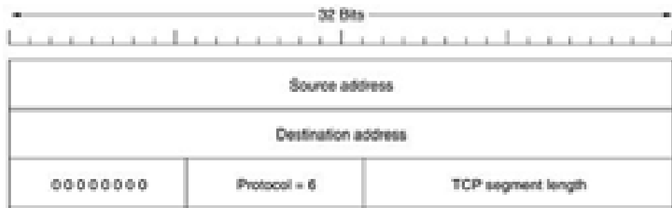
Figure 16-3. The pseudo header included in the TCP checksum.
