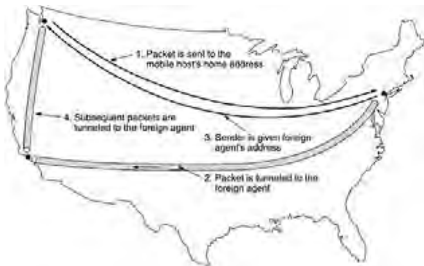
Figure 13-5. Packet routing for mobile hosts.
