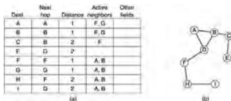
Figure 13-9. (a) D's routing table before G goes down. (b) The graph after G has gone down.
